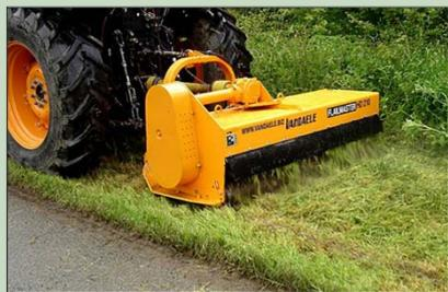
Figure 3. Flail mowers produce fine cuttings that are difficult to remove thoroughly.
