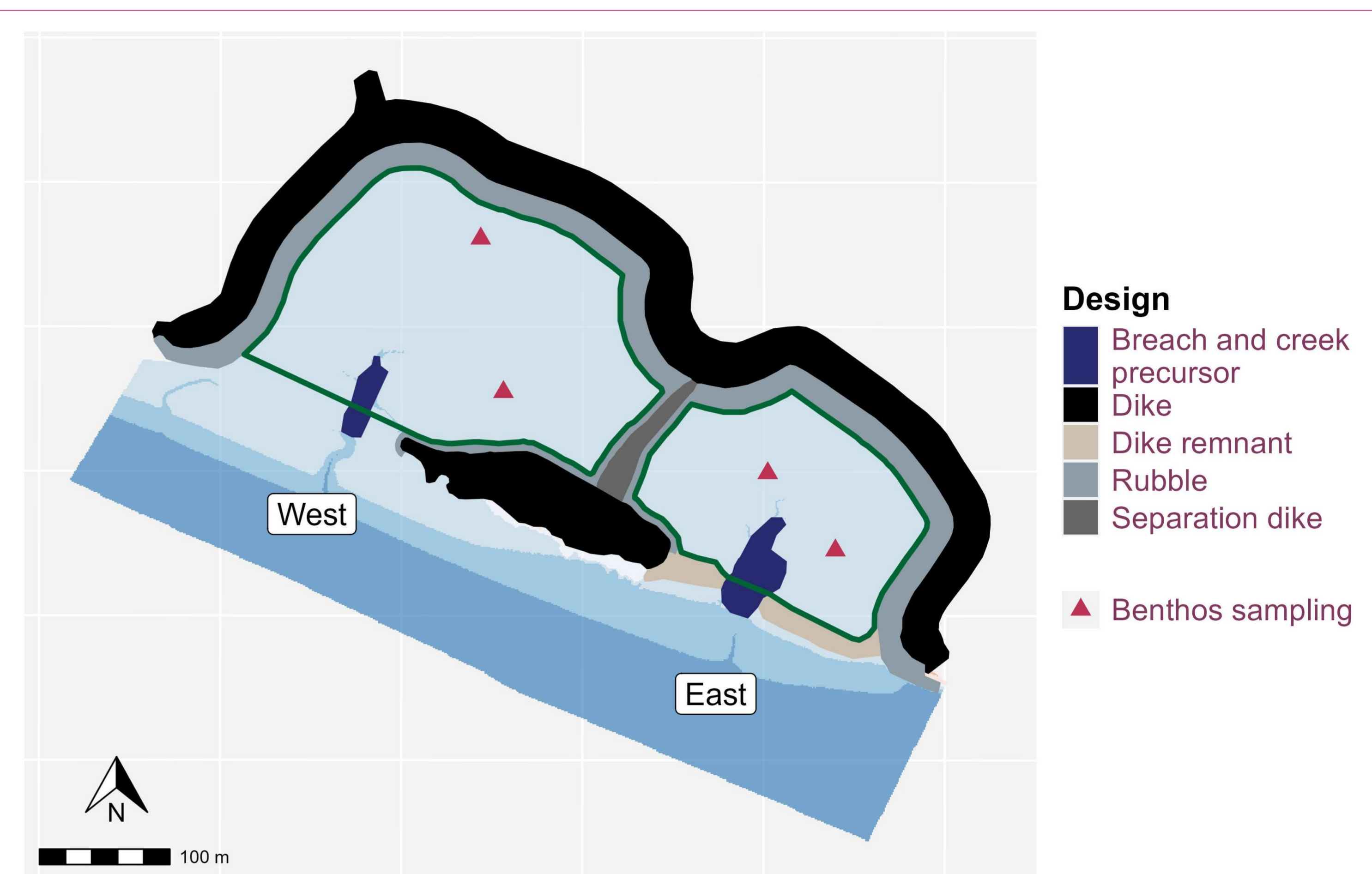
Figure 1: Design of the managed realignment of Lillo's Potpolder. The green line enclosing the compartments highlights the study area.
