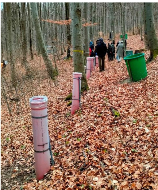
Figure 6-1: Throughfall samplers (left) and stemflow sampler (right) on Level II plot 'Klausen-Leopoldsdorf' in European beech ( Fagus sylvatica ) stand located west of Vienna, Austria. Images: Arne Verstraeten
