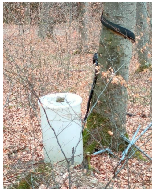
Figure 6-1: Throughfall samplers (left) and stemflow sampler (right) on Level II plot 'Klausen-Leopoldsdorf' in European beech ( Fagus sylvatica ) stand located west of Vienna, Austria. Images: Arne Verstraeten
