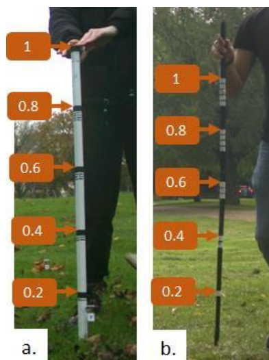
Figure 2. Two examples of calibration poles. The top of each group of bands is at a known height above ground at 20 cm intervals. Heights above ground are indicated in metres, with the number of bands in each group indicating the height increment.
