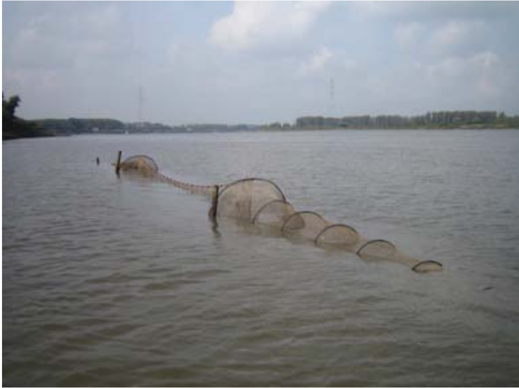
Figure 2.2: Example of a 'paired fyke' net. The net is deployed at the low-tide mark and emptied 24 hours later.
