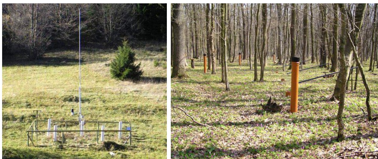
Figure 5-1: Open field (left) and throughfall (right) collectors at an ICP Forests Level II site in Slovenia (Images: Iztok Sinjur and Lado Kutnar, SFI)
