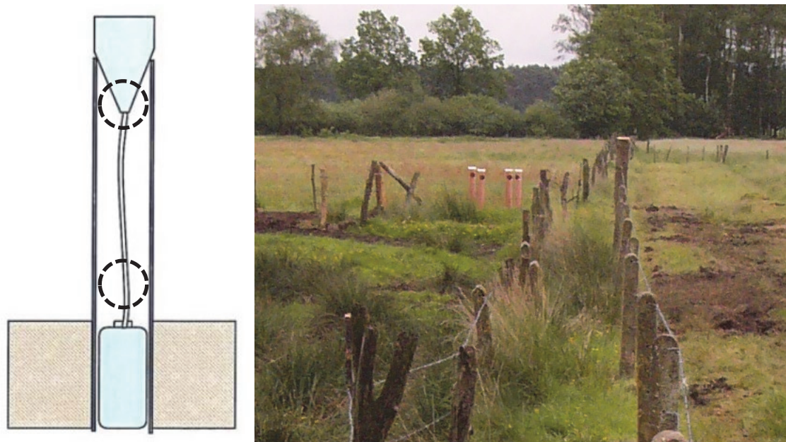
Figure 14 Scheme of a bulk collector and view of the precipitation collectors in the open field near the Level II core plot in Ravels (nr. 14).
