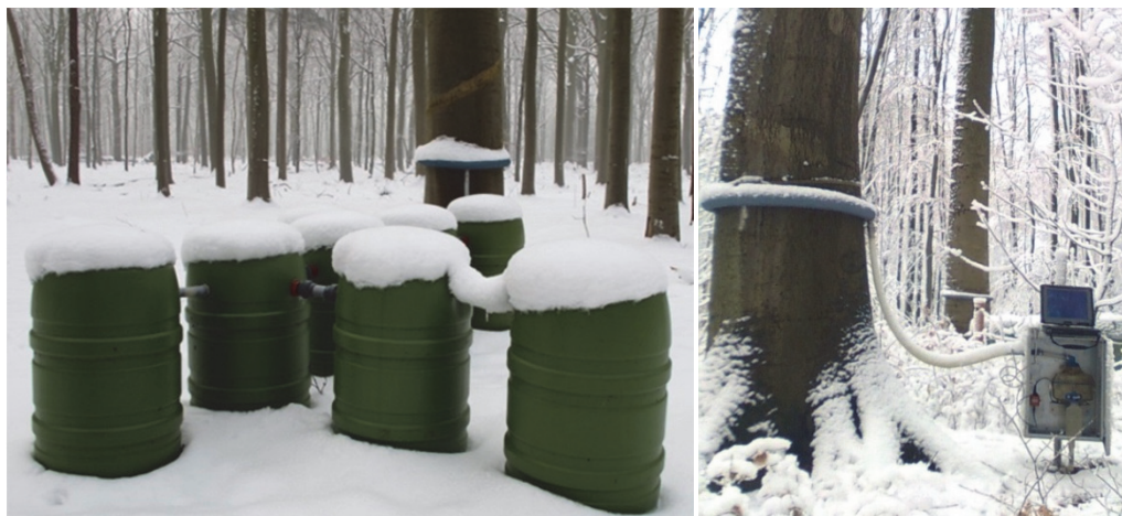
Figure 16 Stemflow collector with containers in the Level II plot in Wijnendale (nr. 11) (left) and with tipping bucket and data logger in the Level II plot in Hoeilaart (nr. 21).
