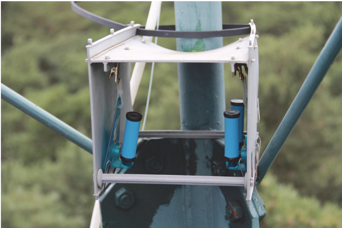
Figure 45 Shelter with NH 3 -passive samplers mounted on a tower rail at 24 m height.
