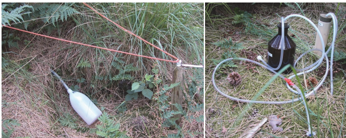
Figure 17 Zero-tension lysimeter (left) and tension lysimeter in the Level II plot in Ravels (nr. 14).
