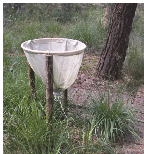
Figure 18 Scheme of the arrangement of litterfall collectors (left) and litterfall collector at the Level II core plot in Brasschaat (nr. 15).
