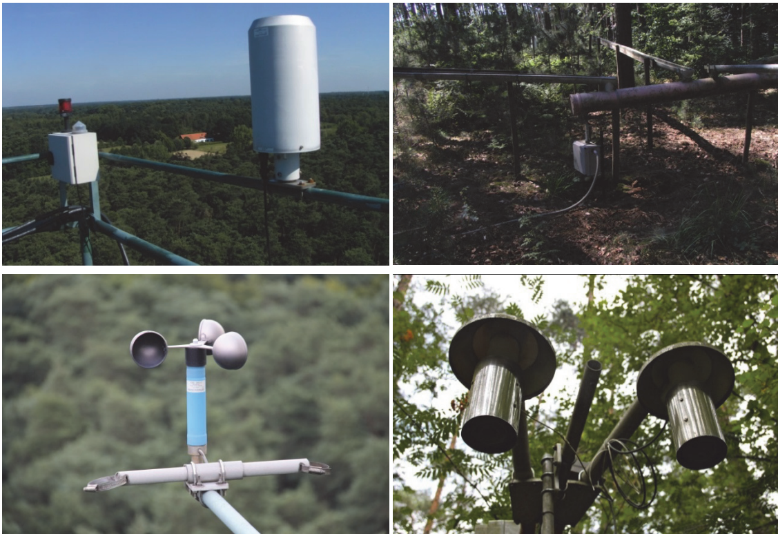
Figure 34 Tipping bucket for rainfall measurement on top of the tower (upper left), gutter system for throughfall measurement (upper right), wind speed anemometer mounted on a boom (lower left) and relative humidity/temperature sensors fixed inside aspirated radiation shields (lower right).
